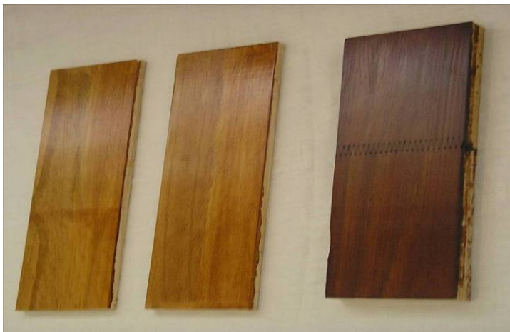
Photo 9: Silverseal stain primer over finger jointed Radiata Pine
