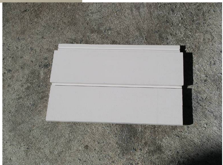
Photo 10: Opaque acrylic paint applied over Silverseal stain primer
